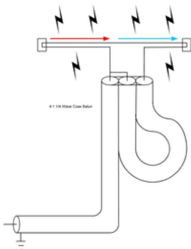
A folded dipole ( $300\Omega$ ) to coax ( $75\Omega$ ) 4:1 balun.
