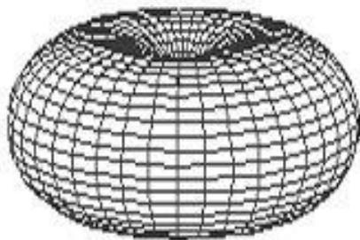
Field strength is maximal in the plane perpendicular to the dipole axis, declining monotonically to zero on the antenna's axis. The 3 dimensional radiation pattern (right) of a vertical dipole is torus-shaped, with equal radiation in all horizontal directions.
