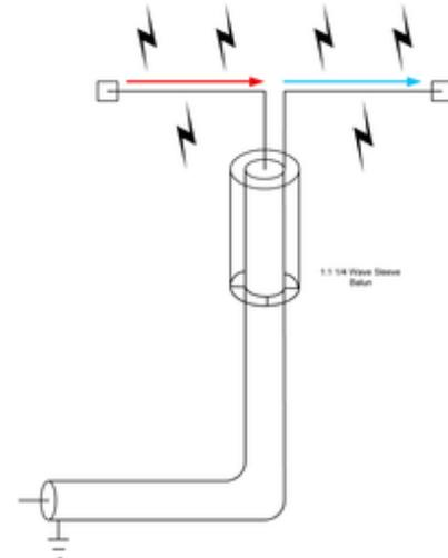
Dipole using a sleeve balun.
