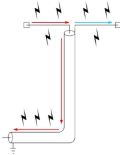
Coax and antenna both acting as radiators instead of only the antenna.
