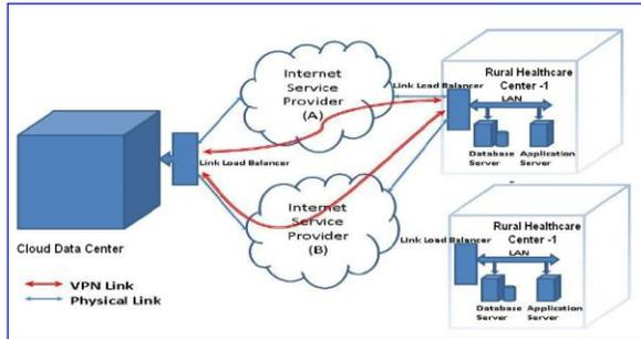
Figure 5(a). Connectivity between Cloud Data Center and Rural Healthcare Centers
