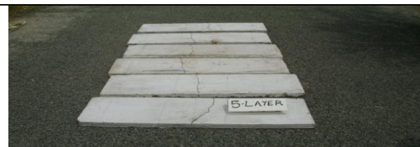
Plate-4 View Of Crack Pattern Of Flexural Plates With 5 Layer Of Wire Mesh
