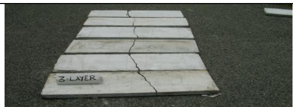
Plate-3 View Of Crack Pattern Of Flexural Plates With 3 Layer Of Wire Mesh
