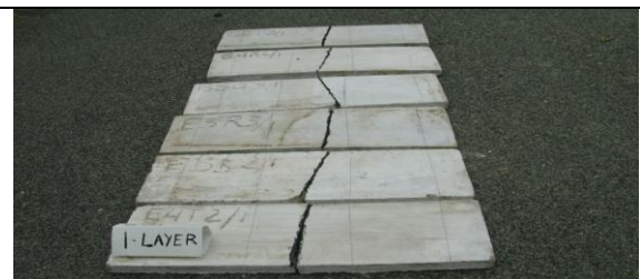
Plate-2 View Of Crack Pattern Of Flexural Plates With 1 Layer Of Wire Mesh
