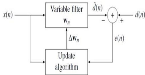
Fig 1. Adaptive Filter Block Diagram
