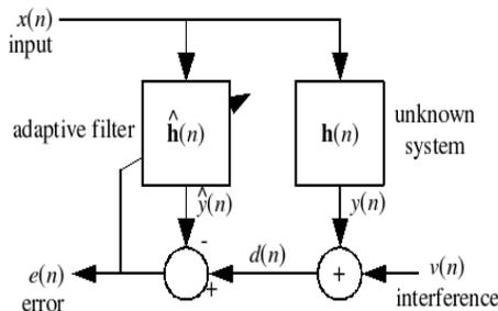
Fig 2. LMS Filter Block Diagram  $h(n)$  is the Impulse Response Of the Unknown System,  $v(n)$  Is Interference)
