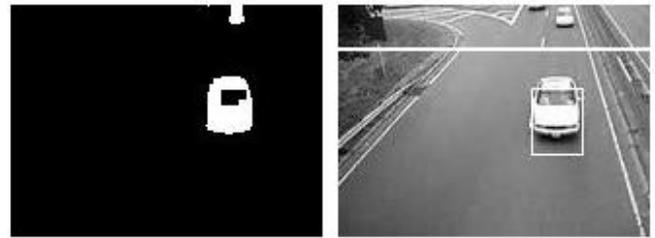
Fig.3. Vehicle detection.
