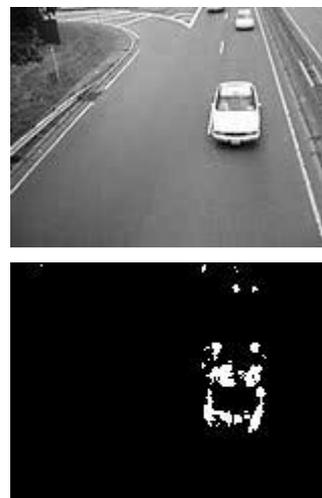
Fig 4. Results of Background subtraction techniques
