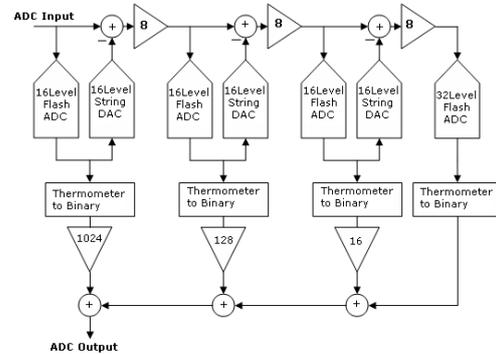
Figure 3.2. Functional diagram of the 14-bit four-stage pipelined ADC
