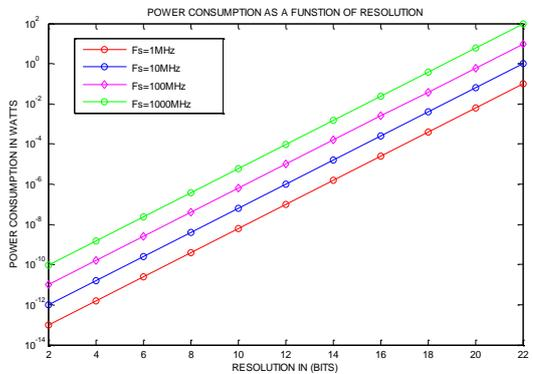
Figure 4.2: Minimum Power Consumption as a Function of Resolution for various Sampling Rate
