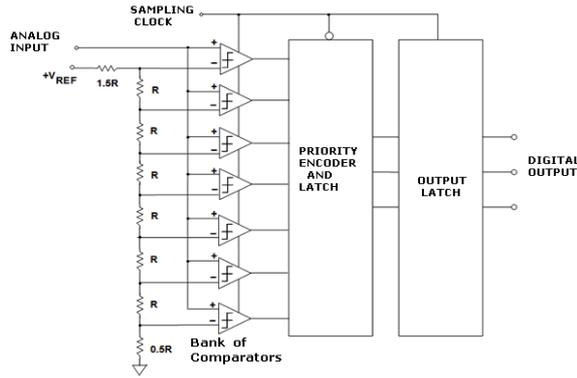
**Figure 1.1: Three-Bit Flash (Parallel) Analog to Digital Converter**
