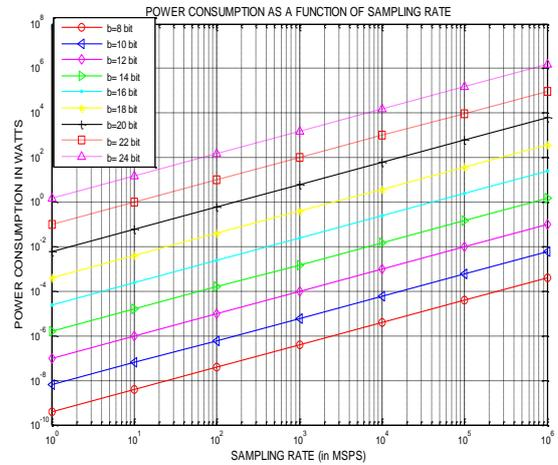
Figure 4.1: Minimum Power Consumption as a Function of sampling Rate for various resolutions
