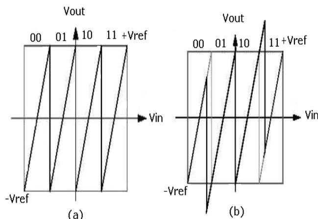
**Figure 3.3: The digital output with respect to the input voltage  $V_{in}$ , (a) Transfer characteristic of a 2-bit stage from the input to the amplifier output in the ideal case (b) with errors affecting the decision levels of the sub-ADC.**
