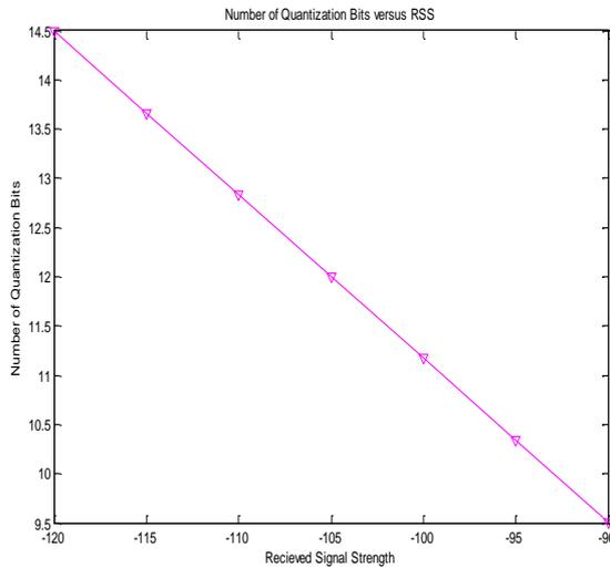
Figure 4.4: Number of Quantization bit as a function RSS
