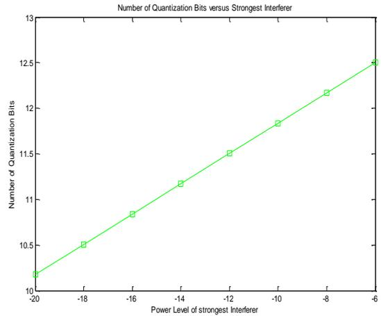
Figure 4.5: Number of Quantization bit as a function of Interference
