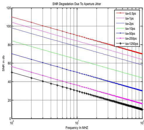
Figure 4.3: SNR Degradation Due to Aperture Jitter
