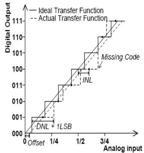
**Figure 2.1: Transfer function of a 3-bit A/D converter [8]**
